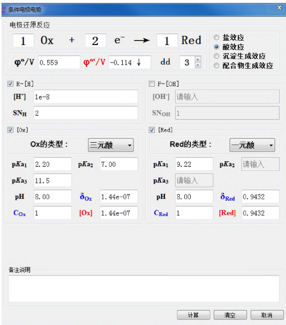
Fig. 6 Estimation of conditional electrode potential for As(V)/As(III) under acidic effect (pH=8.0) 图 6 酸效应下 (pH=8.0) As(V)/As(III) 电对条件电极电势的估算
