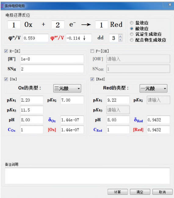
Fig. 6 Estimation of conditional electrode potential for As(V)/As(III) under acidic effect (pH=8.0)
